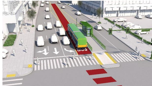
Mixed Traffic: Median Lane
